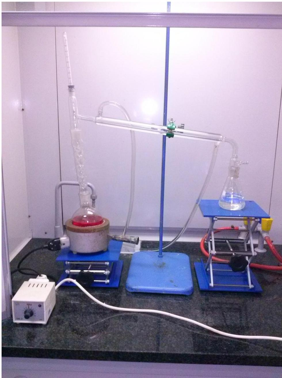
**Analysis.** Weigh precisely 200 ±0,1 g of prepared sample in a clean and dry tared round flat-bottomed flask per 500 cm<sup>3</sup> on a balance (last drops of a sample should be added carefully with a Pasteur pipette). Next add about 30 cm<sup>3</sup> of distilled water. If the analyzed sample is a wine or a mead add additionally 10 cm<sup>3</sup> of 2 M Ca(OH)<sub>2</sub> in the presence of an indicator paper to neutralize the solution. Next add a few glass beads or pumice pieces.
