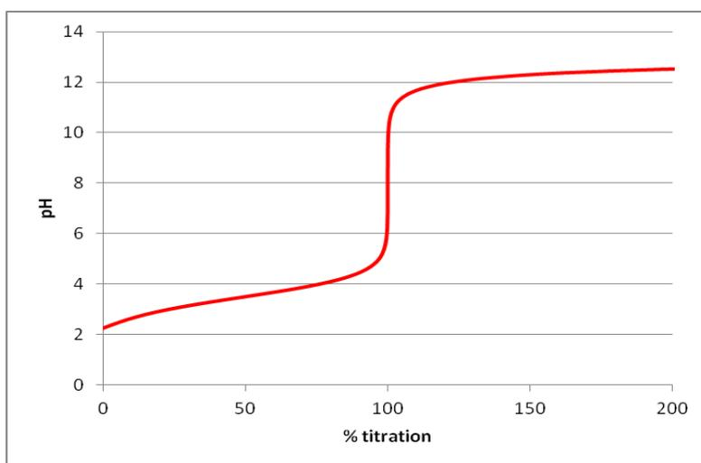
*Titration curve of 0.1 M acetylsalicylic acid using 0.1 M NaOH as titrant*
